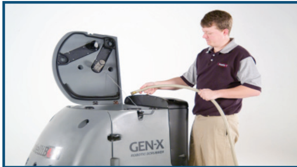
1. The operator fills the GEN-X Scrubber with water and cleaning solution.
