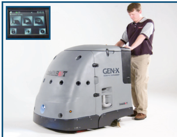
2. The operator selects the desired route on the touch screen and the robot begins.
