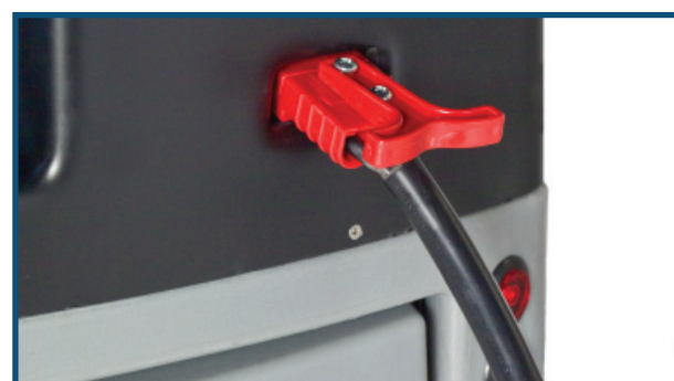
6. The robot is returned to storage and the charger is connected to the battery plug.
