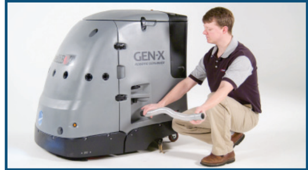
4. After cleaning, the operator extends a hose and opens a valve to drain the tank.
