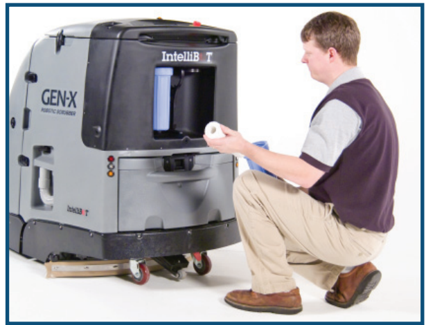
5. The operator unscrews the cartridge filters to replace the cotton elements.
