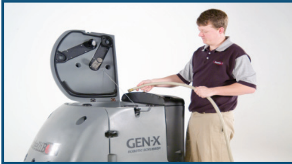
1. The operator fills the GEN-X Sweeper Scrubber with water and cleaning solution.
