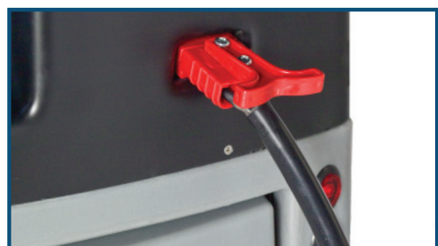
6. The robot is returned to storage and the charger is connected to the battery plug.
