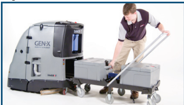
3. If additional run time is required, the operator can exchange the battery pack.
