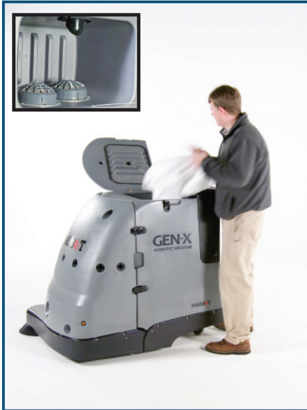
1. The operator installs a clean filter bag and two clean cartridge air filters.
