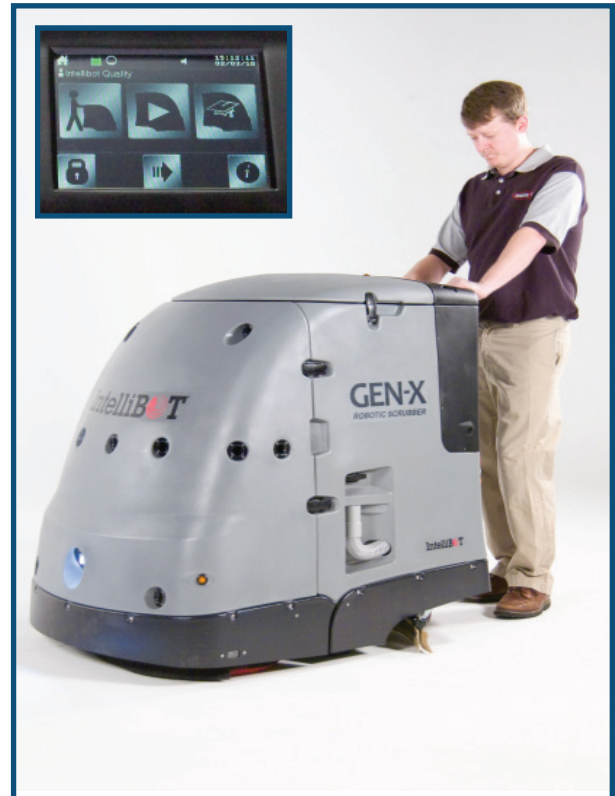
2. The operator selects the desired route on the touch screen and the robot begins.
