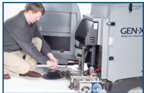
4. Routine maintenance is simple, with unobstructed access to drive belts.
